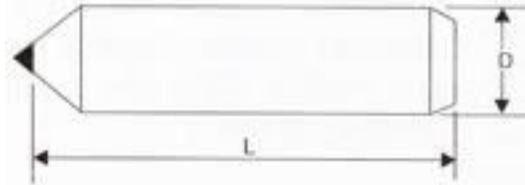
**Details:** Single point "brutted diamond" dressers are made with selected "Congo Rounds" mounted in a matrix. A single cutting edge is presented to the grinding wheel.
